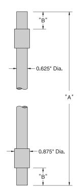
The Elliott Fuse Replacement Bar can be installed in place of a clip mount type current-limiting fuse (that has 0.625-inch diameter ferrels) when a non-fused connection is required. The fuse replacement bar is selected based on fuse mounting codes listed below.
