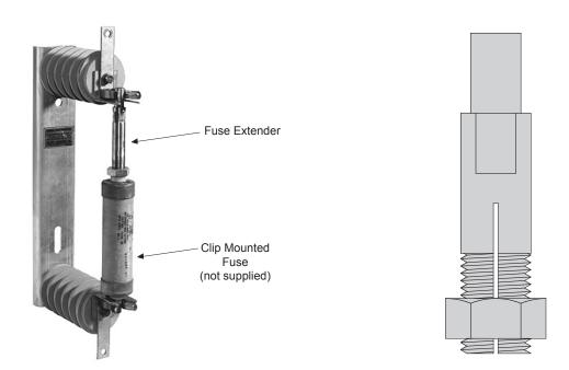
The Elliott Fuse Extender is designed to allow a clip mounted fuse to be placed in a mounting larger than the fuse. For example: a CM5-6 Fuse Extender will allow a Code 5 Fuse to fit switchgear with mountings designed for Code 6 Fuses.
